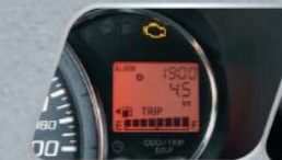
MULTI INFORMATION DISPLAY ECO on/off Indicator, Average/Instantaneous Fuel Consumption, 5 Alarm Settings, Trip Meter, Cruising Range Meter (Tipe G dan TRD S)
