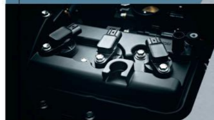
ENGINE 1KR DOHC 12 Valve Electronic Fuel Injection
