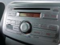
AUDIO 2 DIN integrated audio with CD/MP3/USB/AUX (Tipe G dan TRD S)
